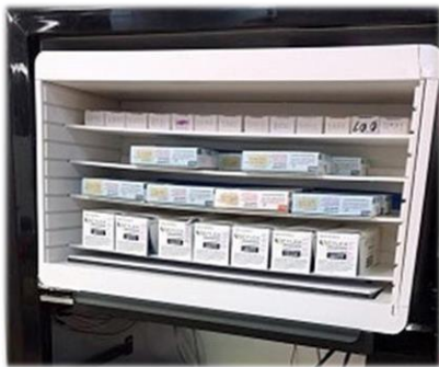
Prototype module to retrofit a refrigerated pharmaceutical dispensing cabinet with an rfidCollect system
